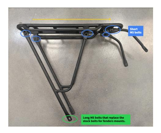
Step 3: Attach the Rack to the Bike Frame
